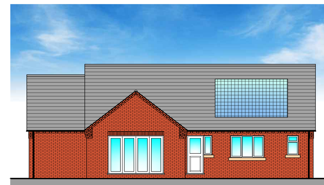
PROPOSED REAR ELEVATION (PLOT 3) (1:100)
